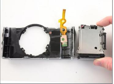
• Remove the battery compartment.
