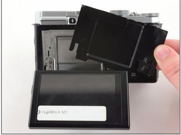
Use two fingers to peel back and remove the black plastic cover from behind the LCD.
