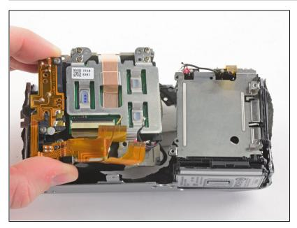
• Remove the sensor assembly.
