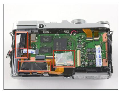
Use tweezers to remove the three pieces of tape covering the components of the motherboard.
