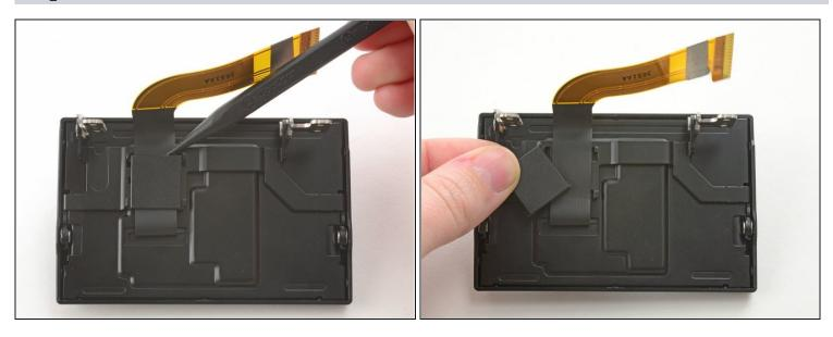
• Use the pointed end of a spudger to remove the ribbon cover on the back of the LCD.
