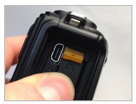
Push the yellow battery/charger compartment tab up using your thumb nail.
