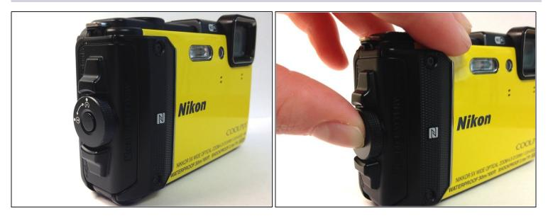
• Using your thumb and pointer finger, open the card/battery hatch by pressing the center button of the wheel and turning the entire wheel to the left.
