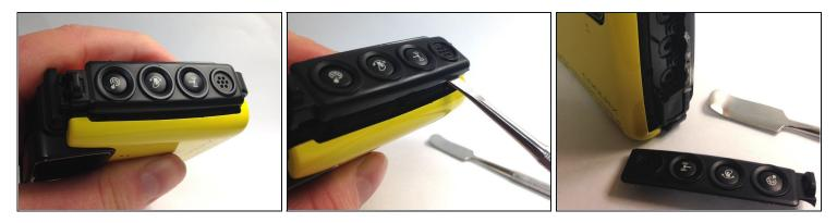
• Using the spudger, pry the plastic button face from the camera body.
