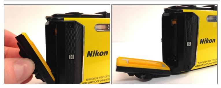
• You should feel the door begin to loosen. Carefully pull the hatch open.
