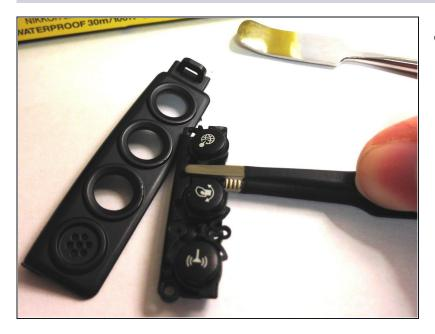
• Using <u>tweezers</u> from the precision tweezer set, remove the buttons from the larger plastic piece.
