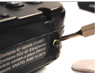
Using a Phillips #00 screwdriver, remove the 2, 4mm screws on the underside of the camera.
