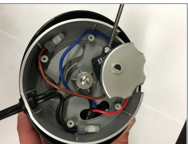
After removing the base of the fan, remove the two screws located under the adjustable speed switch.
