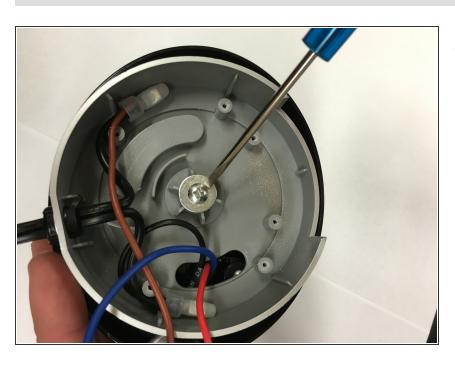
Remove the 4mm screw next to the adjustable speed switch.
