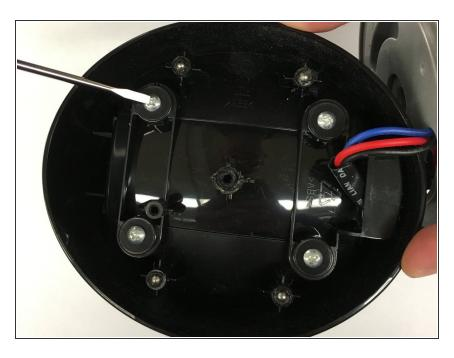
Remove the four 2mm screws.
