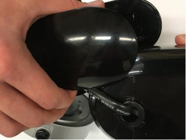
Using two hands, pull the sides out carefully. You will hear a "pop" noise, indicating the sides have came out.
