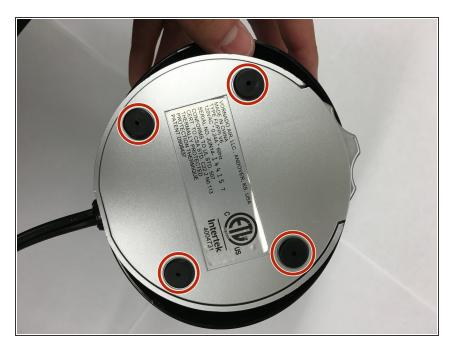
Under the base of the fan, remove the four rubber slip guards by peeling them off with your finger tips.
