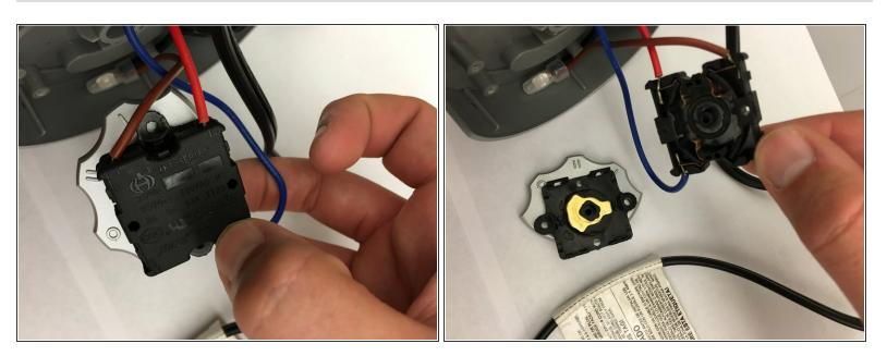
To remove the adjustable speed switch cover, slightly pry off 6 clips located around the switch.
