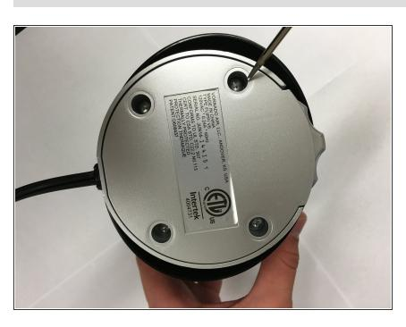
Using the Phillips #1 screwdriver, remove the four 2mm screws underneath the slip guards.
