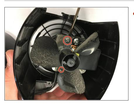
Remove the two 2mm screws holding the blades.
