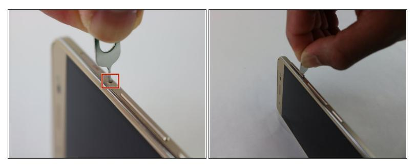
• Flip your device to the right side facing up and use the SIM card eject tool to remove the SIM card by pushing the tool in the hole. You will feel a button click and the tray should slide out 2mm. You will then use your fingers to pull the tray out.
