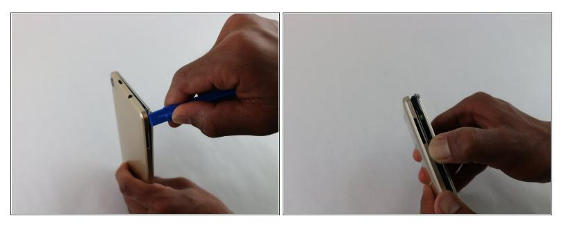
• Take the blue plastic opening tool and insert it in-between the back of the phone and the chrome trim. Go all the way around the device slowly to take the back cover off.
