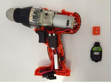
Gently remove the orange plastic speed switch from the drill. It is located right above the motor.
