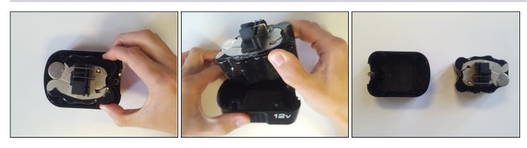
• Grip the battery pack and detach it from the casing by pulling it upward.
