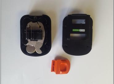
• Remove the highlighted, orange component and set aside.
