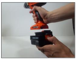
• Detach the battery unit from the drill by pressing down on the battery release button and pulling the battery towards you.
