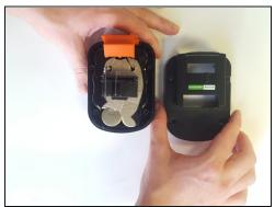
• Now that the screws are detached, separate the two sides of the battery.
