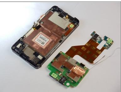
With the back of the main board exposed, flip up the little brown lever at the end of the connector and unplug the final cable that connects it to the main board.
