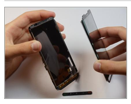
Pop the row of buttons out from the bottom of the phone. They should just fall out when the chassis is off.
