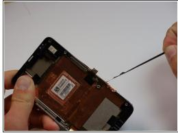
Once heating is done, carfully peel the covering along the sides of the phone away.
