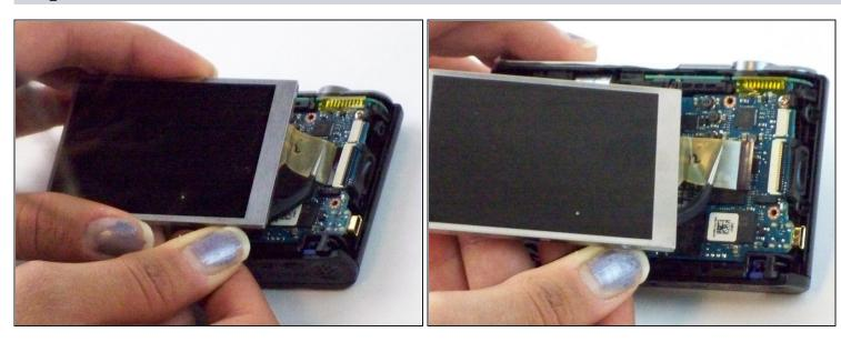
• Gently pull on the ribbon wire disconnecting from the ZIF connector (connecting the LCD screen to the motherboard) with the <u>tweezers</u>.
