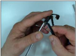
• Carefully put the plastic tool between the glass and the LCD.
