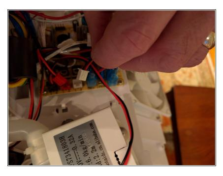
If you have not tested the fans yet, it is recommended that you attach the connector to the fan header on the circuit board, put water in the tank, temporarily re-attach the connector for the ribbon cable to the control panel.
