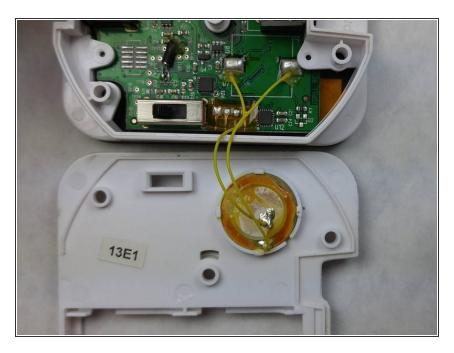
• Desolder the speaker wires from the motherboard.
