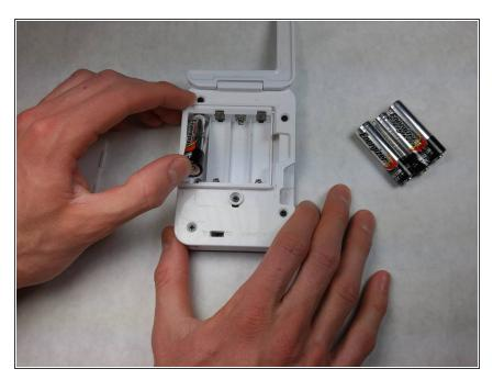
• Remove the batteries from their positions within the device.
