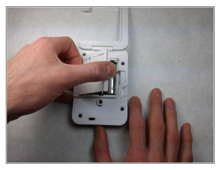
• Remove the plastic cover from the back of the device.
