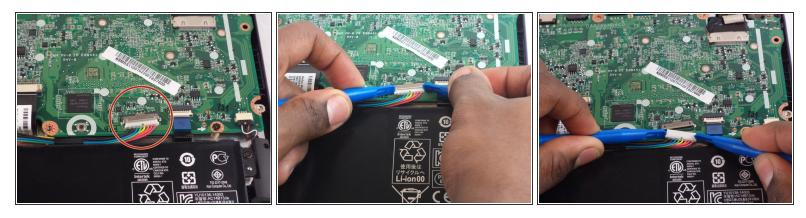
• Using two plastic opening tools tightly grab the connector going from the battery to the motherboard and pull to unplug.
