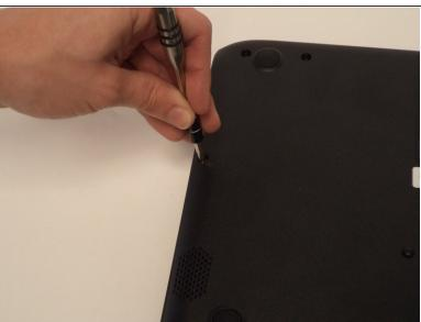
Unscrew the thirteen 6.2mm Phillips #1 screws located on the bottom of the device.
