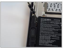
Unscrew two 6.2 mm Phillips #1 screws on the right and left sides of the battery.
