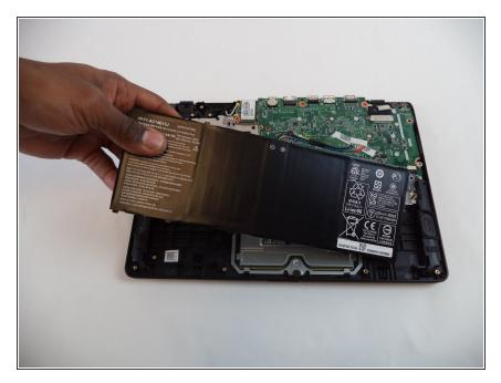
Carefully remove the battery by lifting it out of the casing.
