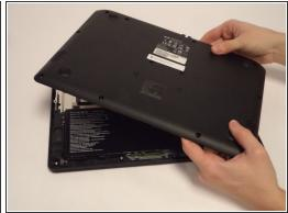
• Lift the back panel using a plastic opening tool. Slowly make your way around the device until the back panel comes off.
