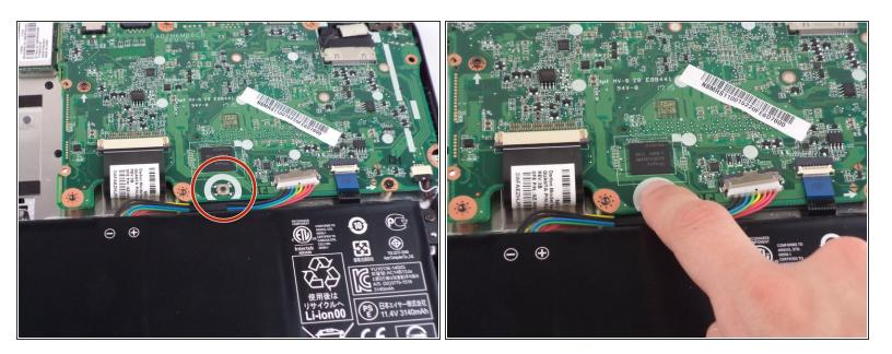
Press and hold the small black button located on the motherboard just above the battery for five seconds.
