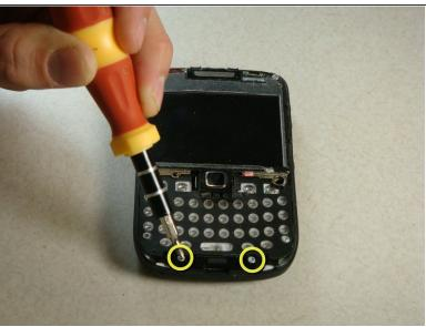
Now there are four screws that need to be removed. They are located at the bottom of the phone and can also be removed using a T6 Torx Screwdriver.
