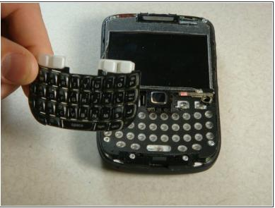
The keyboard should slide off of the phone now that the plastic siding has been removed.
