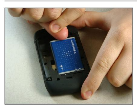
Remove the battery by pulling up from the top of the battery.
