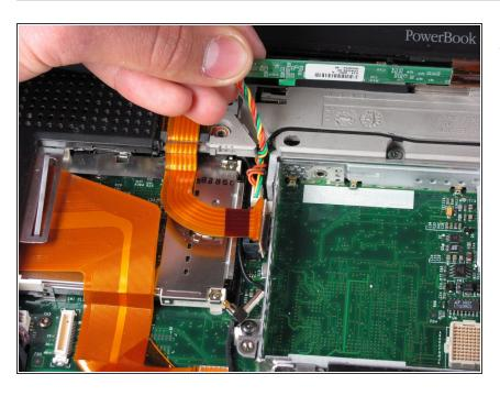
Disconnect the inverter plug by pulling it up from the logib board.
