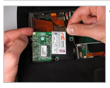
Using your fingers, lift the modem from the socket it is plugged into.
