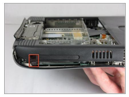
The eject button on the left side of the laptop keeps the upper casing from lifting up. To get around this, you must push the button in to the point that the upper casing can pass by the button and continue lifting up.
