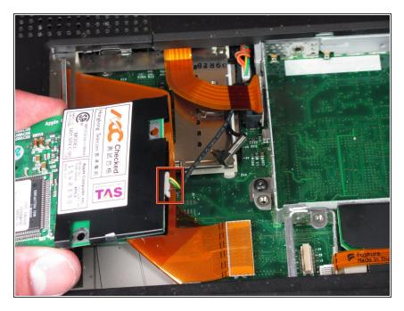
Disconnect the cable that is attached to the end of the modem to remove the modem.
