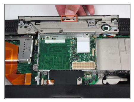
Hold the upper casing in the place shown and pull it back to release the lock. When the lock has released, pull up just enough to keep the case from locking again.
