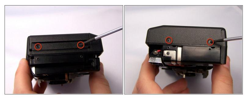
• Remove the two 6.2mm Phillips screws on both sides of camera's back cover.
