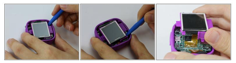
• Use the plastic opening tool to lift the LCD screen, including the purple casing and set it aside, revealing the motherboard and connector ribbon.
