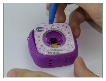
Pry off the transparent plating and paper design using a plastic opening tool.
