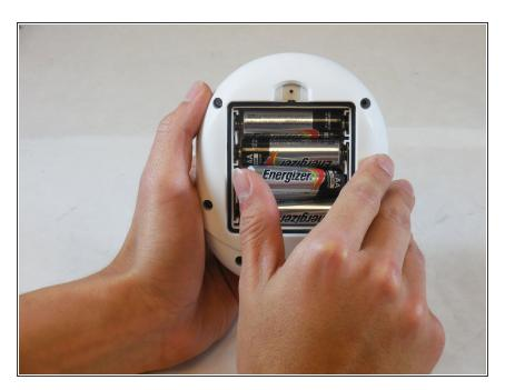
Remove and set aside the (4) AA batteries in the battery housing.
