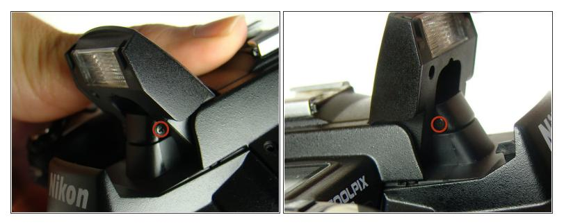
• Remove the Phillips screws on both sides of the flash bulb mount.
