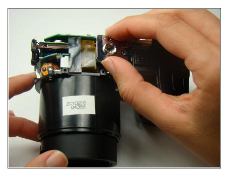
• Remove the silver tripod mount by sliding it towards the speaker.
