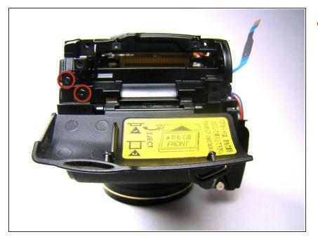
Remove the two Phillips screws located underneath the CF card cover.
