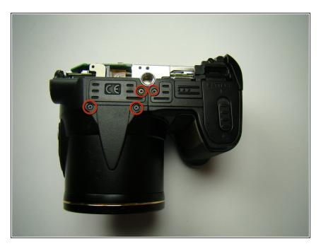
• Remove all four of the screws on the bottom of the camera.
