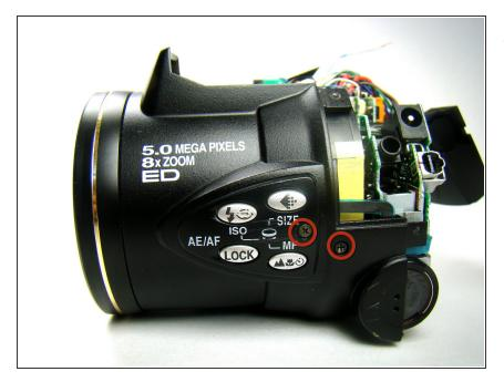
• Remove the two screws on the left side of the camera.
