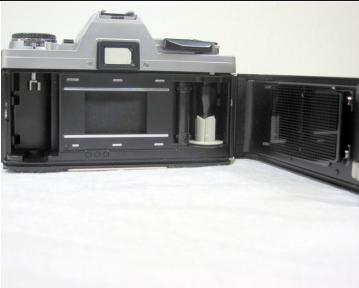
• Lift up the winding lever and rotate it clockwise to open the back film compartment.
