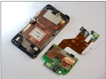
With the back of the main board exposed, flip up the little brown lever at the end of the connector and unplug the final cable that connects it to the main board.
