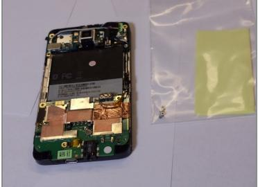
• Remove five T5 Torx screws from the motherboard.
