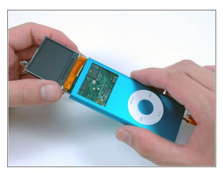
Completely remove the display and logic board from the iPod.
