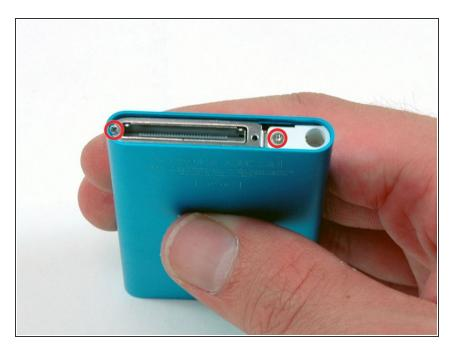
Remove the two Phillips #00 screws from either side of the dock connector.
