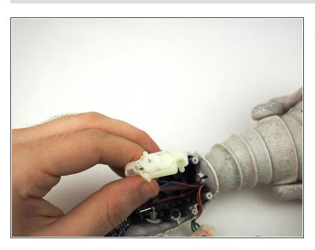
Inspect the gears inside the assembly and replace any gears that have flattened or rounded teeth.
