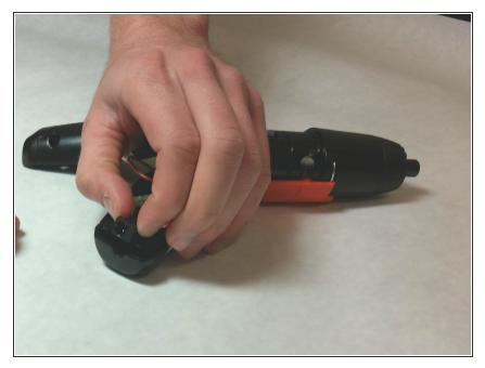
• Pull the charging port and circuit board away from the casing.
