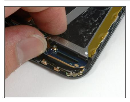
There is a copper rim on the small antenna connect board that contacts the antenna.
