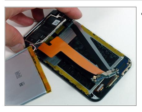
Lifting the logic board up to see what's beneath.
