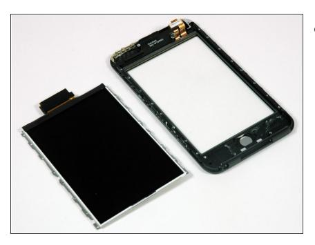
The touch-screen LCD on the left, and display bezel on the right.
