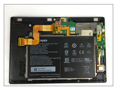
Locate the cable that is connecting the camera to the tablet
