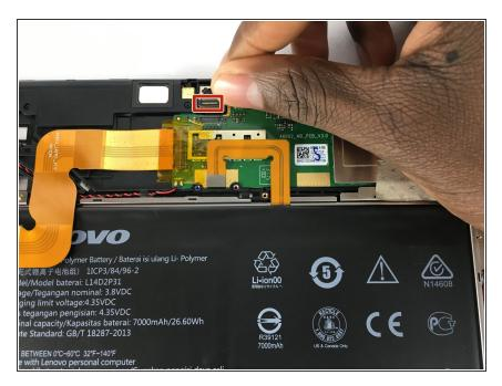
Disconnect the cable that is connecting the camera to the tablet
