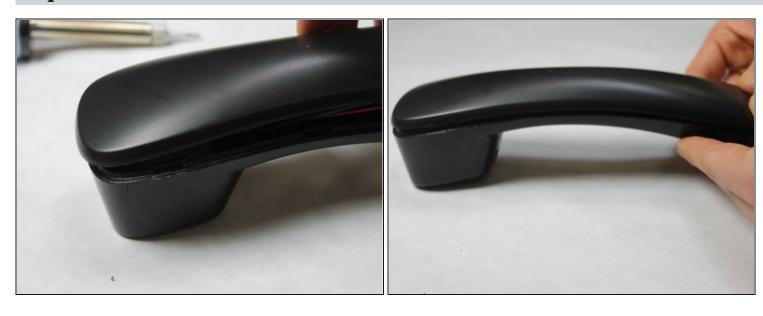
• Continue separating the two sections by using the metal spudger all the way around the edge of the handset.
