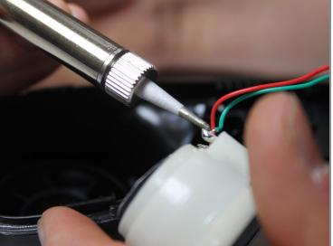
• Use a soldering iron to melt the existing solder off of both the red and green wires in order to completely remove the speaker.
