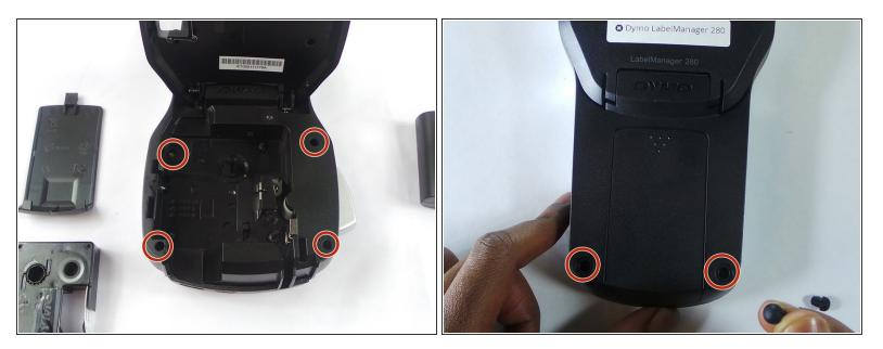
Remove the 6 screws in the indicated places. These particular screws are 2mm x 8mm Phillips #0 head
