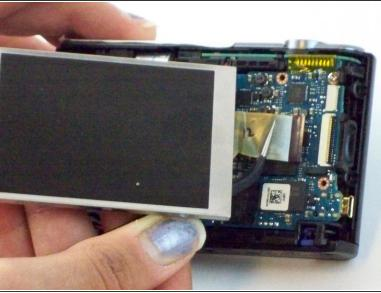
Gently pull on the ribbon wire disconnecting from the ZIF connector (connecting the LCD screen to the motherboard) with the tweezers.
