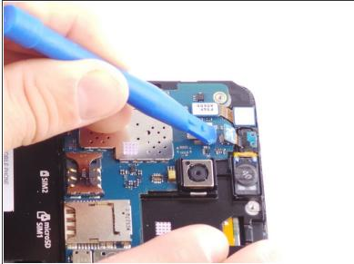
Use the plastic opening tool to unhook the ribbon cable clip.
