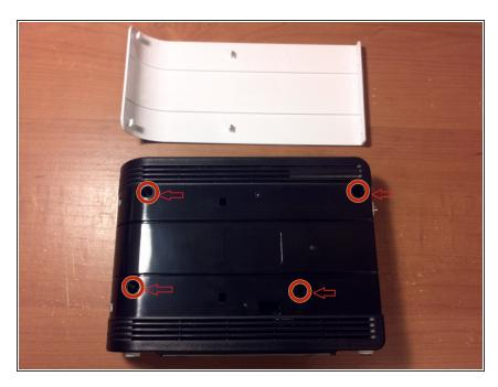
Locate and remove the four Phillips screws
