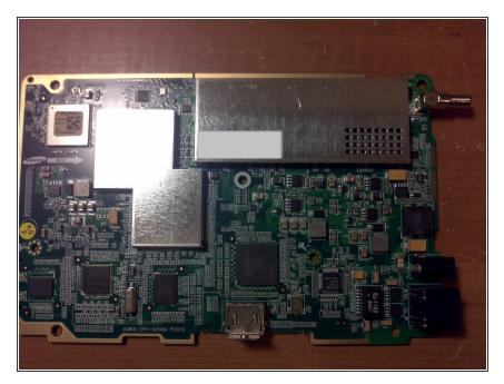
Using an 8mm socket you can remove the antenna pigtail.
