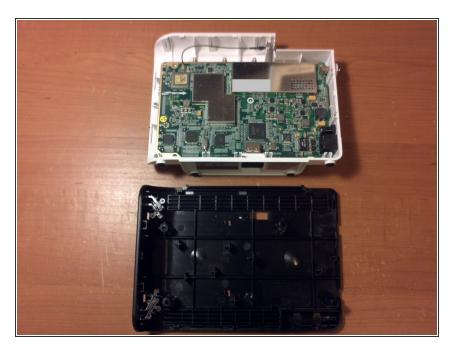
With the cover removed you now have access to the circuit board.
