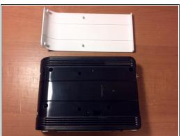
Use a pry tool to remove the white outer cover. Pry towards the front of the device. Continue prying down the length of the cover until it pops off.
