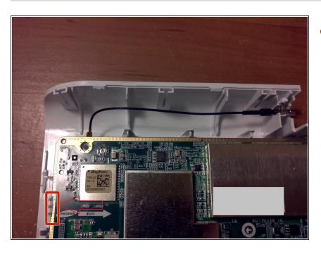
Release the clip indicate to remove the circuit board.
