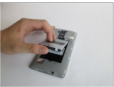
Insert the plastic opening tool into the indent at the bottom of the battery and lift up. Fully remove the battery with your fingers.
