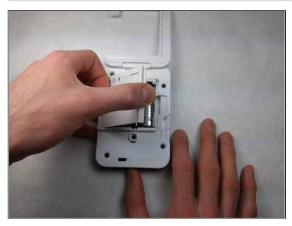
Remove the back plastic cover from the device; this should allow you access to the batteries.
