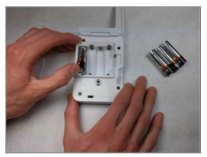
Remove the batteries from the device.
