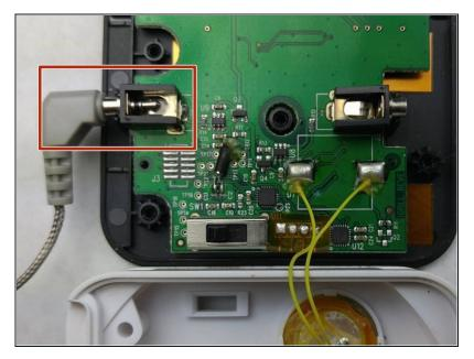
Using a pair of tweezers, bend the probe contacts back in place. The tweezers will touch the probe terminals when inserted.
