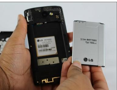
Use the thumb tab to remove the battery.
