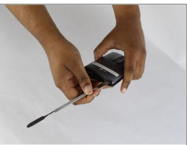
Slide a plastic spudger, or guitar pick, between the back and front panel at the bottom.
