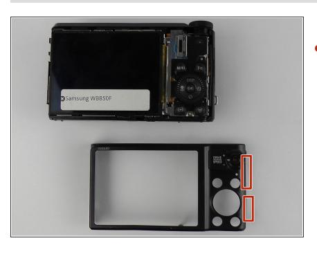
Once the screws are removed, use the blue opening tool to open the back case from the sides - it should come off easily.
