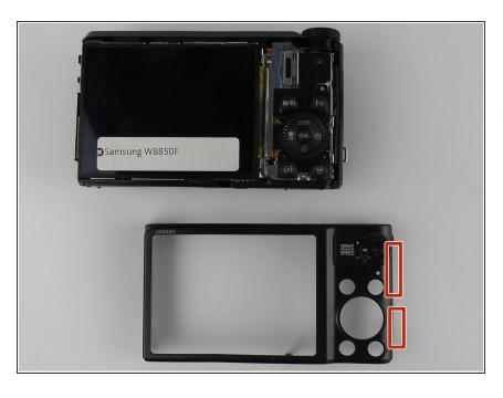
To remove the back screen case, use the blue opening tool to open the case up from the right side.
