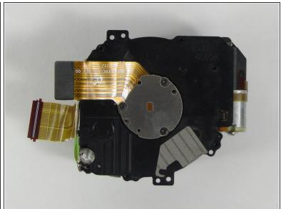
Gently pull up on the lens connector chip to remove the lens.
