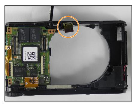
Insert the new lens to be replaced.
