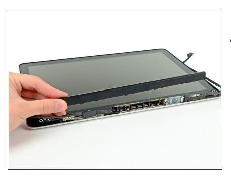
Remove the clutch cover from the display.
