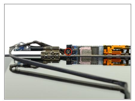
Remove the single 3.3 mm Phillips screw securing the camera cable retainer to the display.
