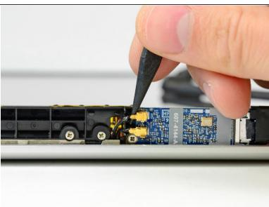
Use the tip of a spudger to pry both AirPort antenna connectors out of their sockets on the AirPort board.
