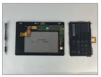
Once the battery ribbon cable is detached, carefully remove the battery.
