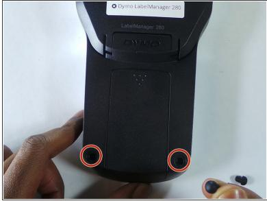
Remove the 6 screws in the indicated places. These particular screws are 2mm x 8mm Phillips #0 head
