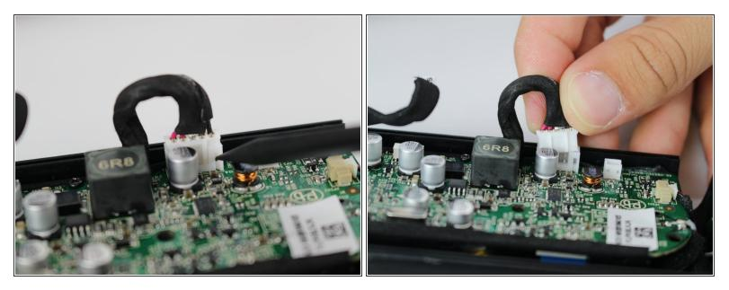
• Using the black spudger, carefully remove the cord connecting the battery to the motherboard.
