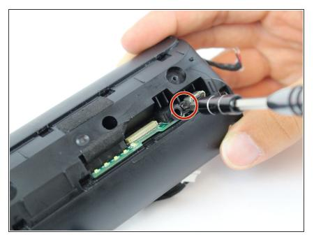
Remove the 7.0 mm Philips #1 screw that connects the I/O board to the casing.
