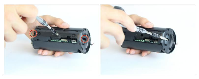
Using the driver adapter, first insert the #4 socket into the driver; followed by the #1 Philip's head bit in order to reach the three 13.0 mm screws.
