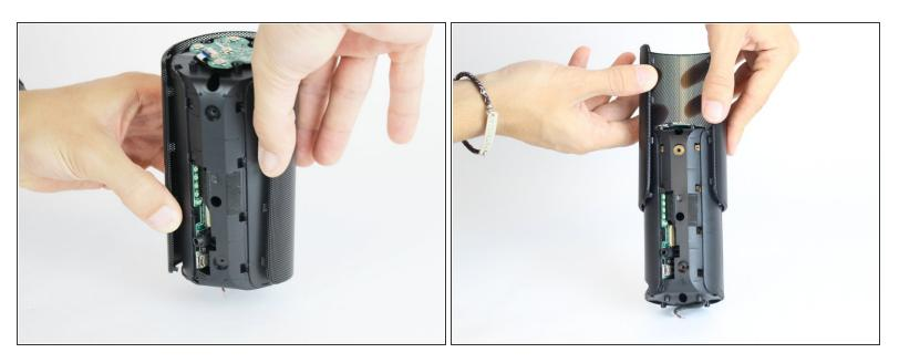
• Expand the metal casing and carefully slide it off the speaker.
