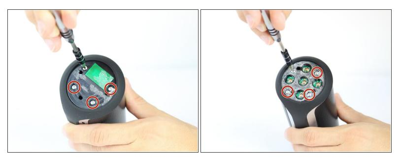
• Remove the eight 7.0 mm Phillips #1 screws on both sides of the JBL Flip 2.
