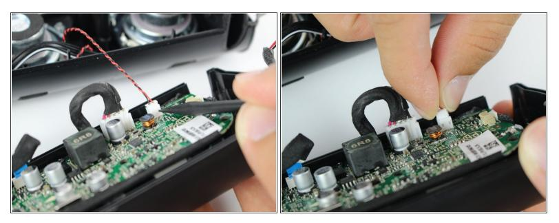
• Use the black spudger to disconnect the auxiliary wire from its socket.
