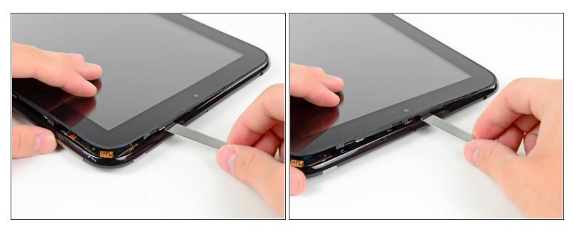
Pry up the front panel assembly along the top edge of the TouchPad.
