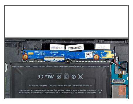
Remove the two 3.0 mm Phillips screws securing the digitizer control board to the rear case.
