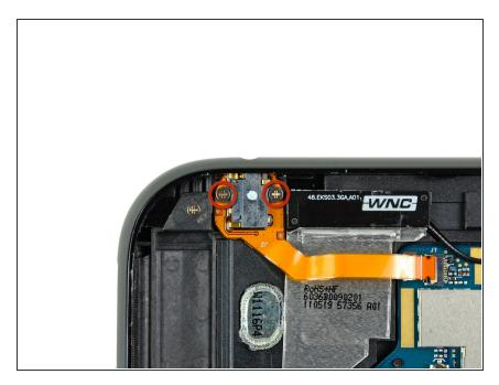
Remove the two 4.4 mm Phillips screws securing the heaphone jack to the rear case.
