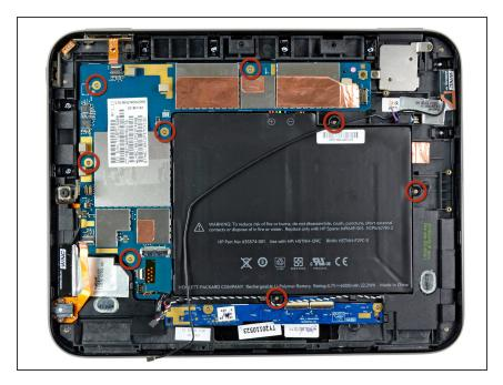
Remove the eight 3.2 mm Phillips screws securing both the battery and the motherboard to the rear case.
