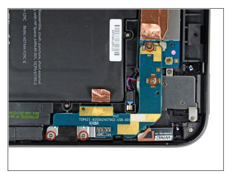
Remove the four 3.2 mm Phillips screws securing the USB connector board to the rear case.
