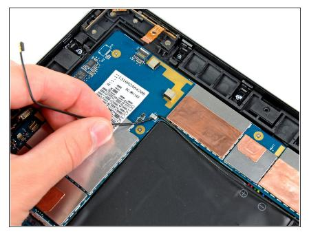
De-route the lower antenna cable along the top edge of the battery and carefully pull it out from under its retaining clip near the top right corner of the battery.
