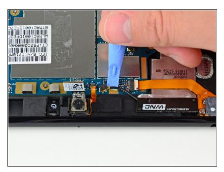
Use your plastic opening tool to pry the upper antenna connector up from its socket on the motherboard.
