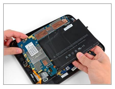
Lift the motherboard assembly out of the rear case, minding any cables that may get caught.
