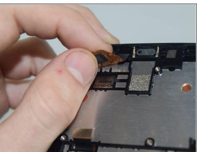
Using the plastic opening tool, pry the display cable from the body of the phone.
