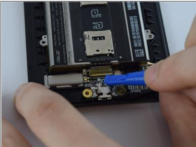
Using the plastic opening tool, unlock the ribbon cable attaching the battery to the circuit board by prying up the yellow tab.
