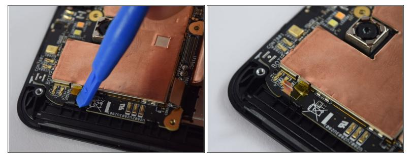
Using a plastic opening tool, disconnect the display cable from the side of the motherboard by carefully sticking the tool underneath the display cable and gently pulling outward.
