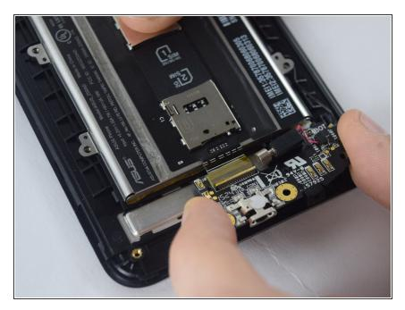
Gently remove the circuit board from the phone by gently pulling it away from the bottom of the phone.
