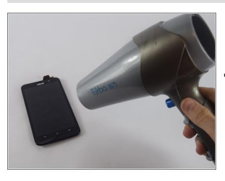
Using a hair dryer or a heat gun, heat up the adhesive that attaches the display to the housing. The
