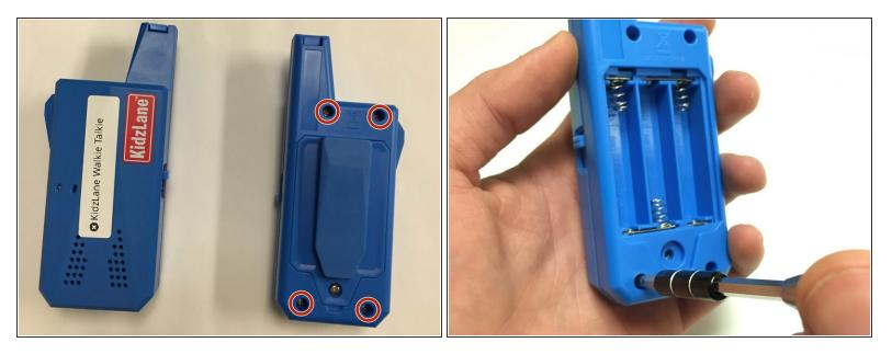
• Use a screwdriver to remove the four pictured 4mm screws.
