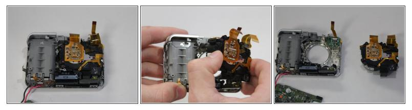
• Grasp the lens assembly and carefully lift it out of the camera.
