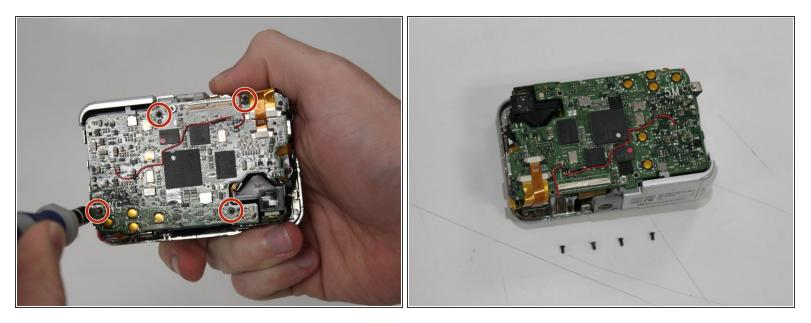
Locate four black 3.0 mm screws on the motherboard and remove them using a Phillips screwdriver with a #0 bit.
