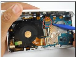
• With the screen freed, gently lay the camera on its face, so that the battery compartment faces up. Use both hands to lift the screen up and away.
