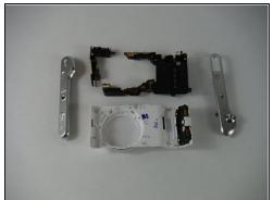
• Next, gently use the plastic opening tool to pry the black frame out of the casing. The frame should lift out easily. If you feel some resistance, you may have missed a screw.
