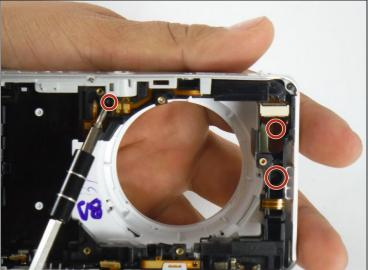
• Now, all that's left is the frame and black interior frame. To get to the flash assembly, the black frame must be entirely removed.
