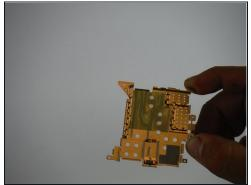
Underneath the motherboard, there is a thin metal plate. This plate should lift up easily, as there are no screws keeping it in place.
