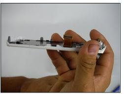
• With the screen separated from the main chassis, use the plastic opening tool to gently pry the edge of the ribbon cable connector from the motherboard.
