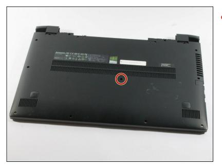
• Remove the one (40 mm) screw in the middle of the Flex 15.
