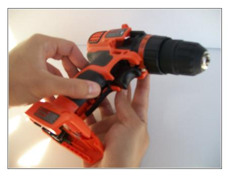
Gently grab both sides of the drill casing, and separate both sides from each other.
